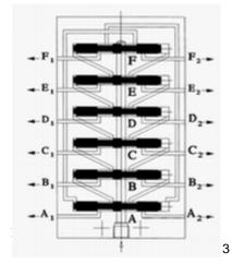
When lubricant is supplied to the main line connection of the progressive distributor, piston "A" (for instance) is moved in direction of outlet A1 up to the limit stop is metered to outlet F2. The delivery of lubricant is continued and piston "B" is moved in direction of outlet B1up to limit stop, and the lubricant in front of the limit stop is carried to outlet A1. In the continued succession, piston "C" is moved in direction of outlet C1 up to the limit stop,
